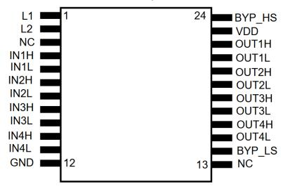
3.9 mm×8.65 mm; Thickness,1.45mm; Pitch, 0.635 mm
